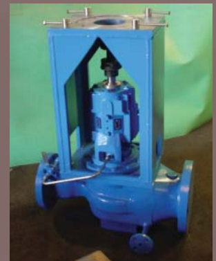
Modified using a Goulds SX Standard Bearing Frame
